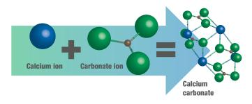
All Physical Water Conditioners endeavour to create the same non-chemical effect for control of the scale. They generate a seed / nucleation point that attracts the elements that produce scale and holds them in suspension. This prevents the hardness minerals from forming on the internal surface areas of the water system, and are instead allowed to flow through the water system and out to drain.
