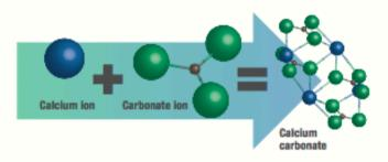
All Physical Water Conditioners endeavour to create the same non-chemical effect for control of the scale. They generate a seed / nucleation point that attracts the elements that produce scale and
